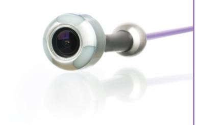
Stainless steel and epoxy resin enclose the glass covering the lens of the K-28 HD and make it robust. Thanks to the flexible yet hard-wearing end piece, it can be used in pipes from DN 40 and up, making it ideal for use in bathrooms and kitchens.
