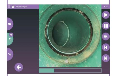
After completion of the inspection, the survey is saved in a project folder on the removable disk, along with the corresponding photos. The files are saved in the formats jpeg (images) and MP4 (videos) and can therefore be opened and played on all PCs. If reports are to be created, an import to can3D® is possible.
